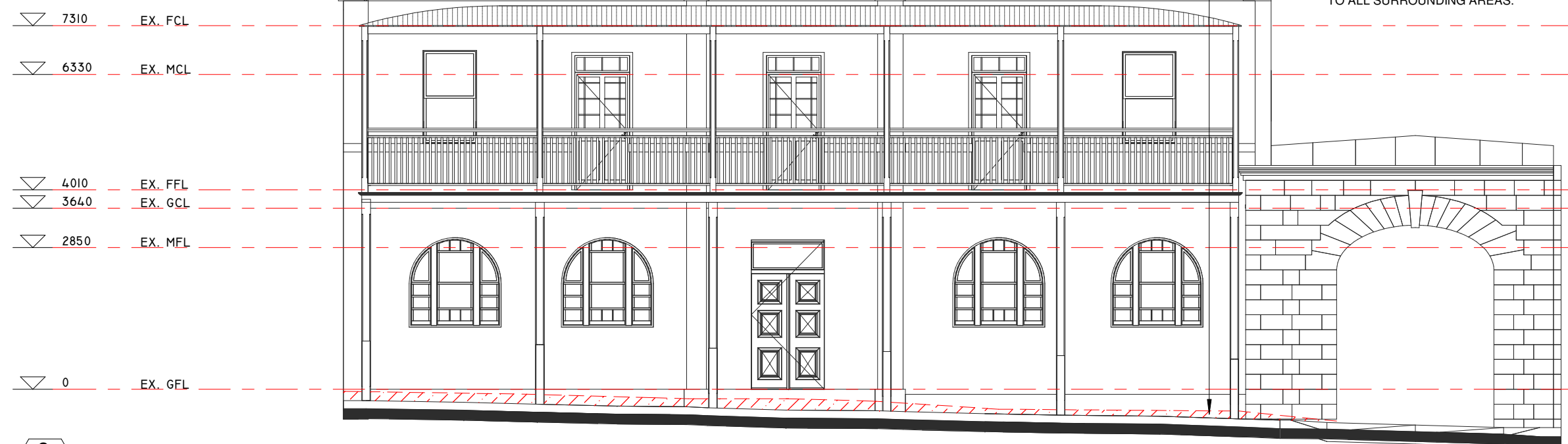
2 DEMOLITION SOUTH ELEVATION 1 : 100 @ A3
